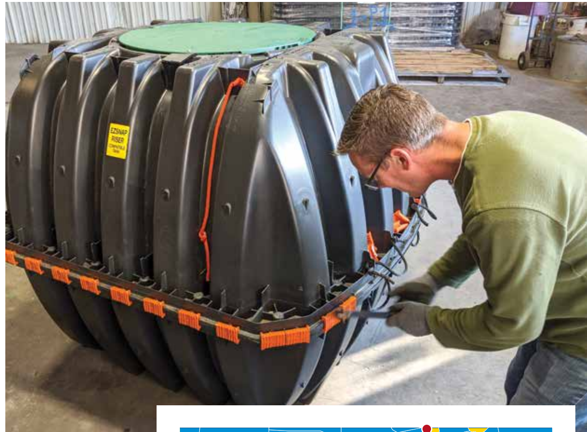
▼ Anderson assembles an Infiltrator Water Technologies IM-540 tank. (Photo by Ray Tebo)
